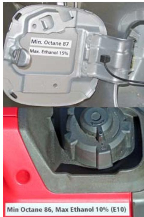
Filler cap labels for vehicle and generator.
