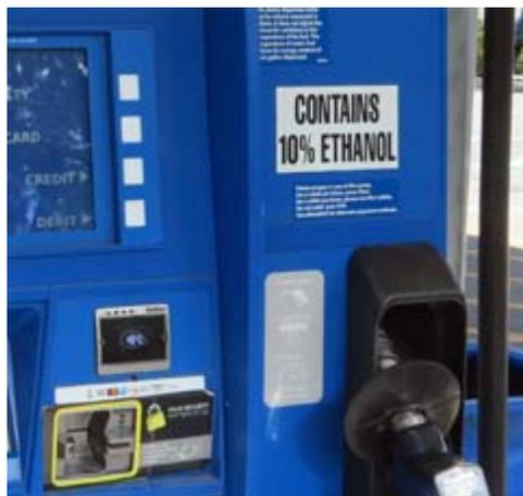
Mobil gasoline pump is clearly labeled with percentage of ethanol.
